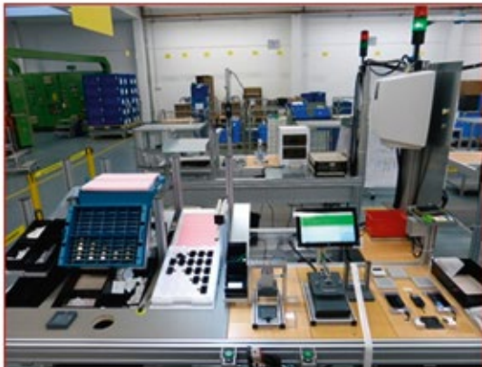
1. Assembly of “control module” including functional testing
